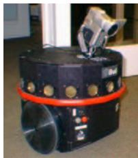
Figure 1: Nomad Scout II Robot with Vision System
