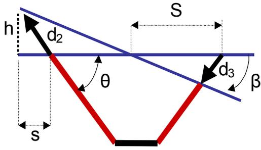
**Figure 11.** Correlation between the pistons 2 and 3 displacement ( $d_2$  and  $d_3$ ) and the tilt of angle  $\beta$  is
