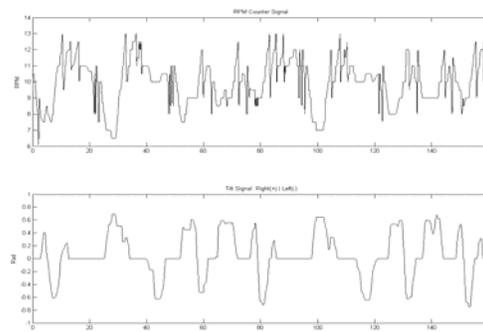
Figure 6. Motorcycle acceleration/braking and tilt data respectively calculated from video
