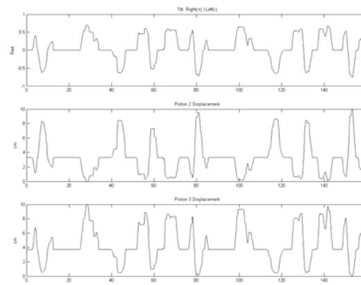
Figure 7. The tilt data and resulting displacement data of piston 2 & 3 respectively
