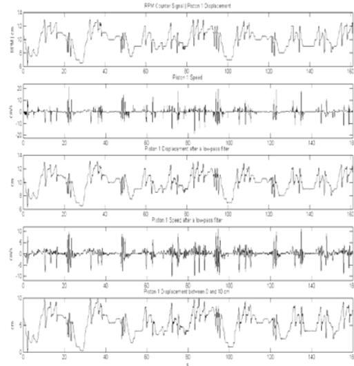
**Figure 9.** Graphs showing piston 1 displacement and corresponding speed with filtering
