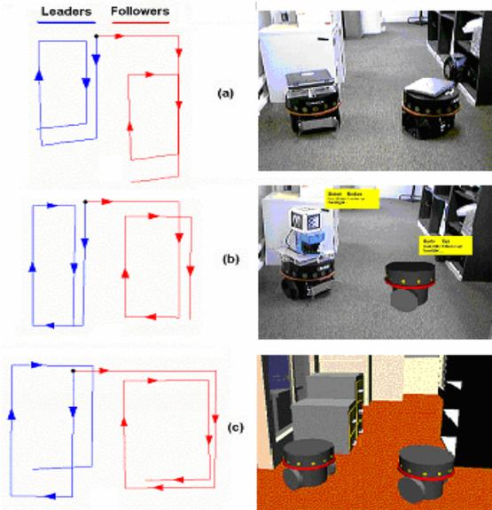
Fig. 8: Trajectory traces (left) and pictures (right) for few steps of the Waltz task. From top to bottom: (a) Full real experiment, (b) Real leader and simulated follower, (c) fully simulation dance.
