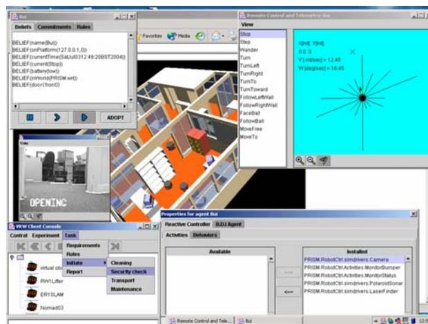
Fig. 3: Workbench Applet GUI (from upper left clockwise: BDI debug window, telemetry and tele-robotic panel, BDI property dialogue, Workbench console with task/role management and acquaintance list, RTP video feedback, 3D view in background).
